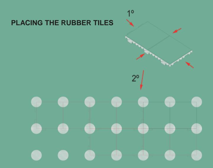
FIRST, apply the adhesive through the cannula, on the side surfaces of the tiles. Then join against the adjacent faces. The surfaces must be in contact with each other in a forceful way, to ensure a correct gluing.
