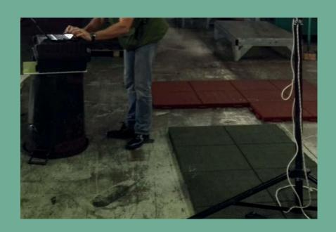
FLEXIFOR tiles from SBR (recycled wheels) together with first generation resins. They are pavements suitable for different applications such as absorbent surfaces of playgrounds, surfaces for gyms, terraces, stables for horses and other animals, as well as for shooting galleries and insulation surfaces.
